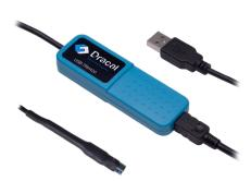
The TRH200 is designed for environmental temperature and humidity acquisition. Its exposed sensor allows a more precise temperature measurement of hard surfaces. The TRH320 is field interchangeable, thanks to its factory calibrated, linearized and temperature-compensated digital sensor chip. With its precision electronics, extremely small variations in temperature and humidity can be detected.
